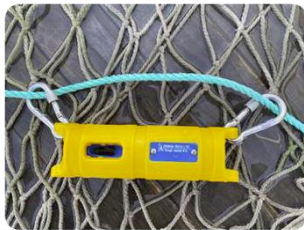
Alternate attachment for trawl, directly to the net using a lead rope.
