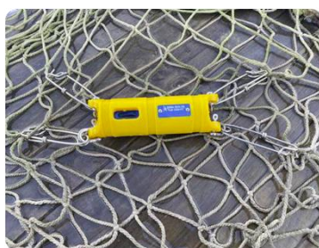
Moana sensor in tough jacket #3 directly attached to a net or weaved in.
