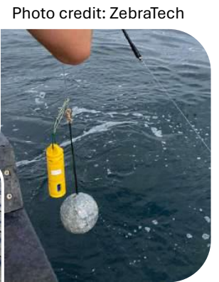
Moana sensor attached to anchors using either tough jacket #3 or tough jacket #4.
