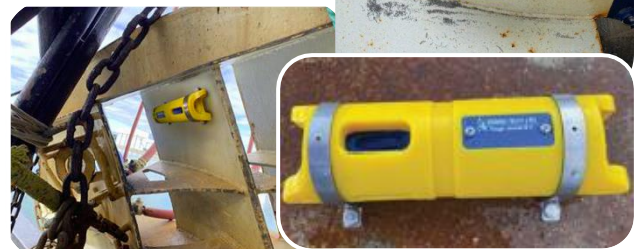
Moana sensor attached to trawl door using tough jacket #3 and brackets.
