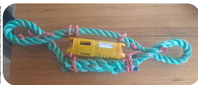
Moana sensor in tough jacket #3 directly attached to a net or weaved in.
