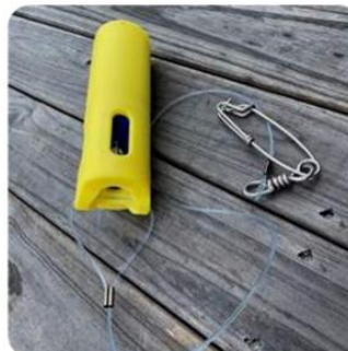
Moana sensor in tough jacket #4 attached to a shark clip / clasp to be attached to the middle of a set on a longline.
