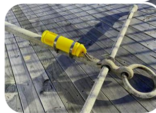
Moana sensor attached to anchors using either tough jacket #3 or tough jacket #4.
