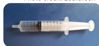
Equipment for testing the Moana sensors: rope, monofilament and sinker, or a small plastic syringe.
