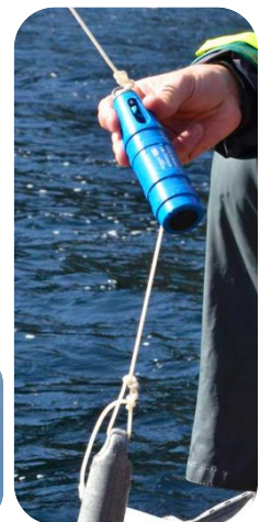
Equipment for testing the Moana sensors: rope, monofilament and sinker, or a small plastic syringe.
