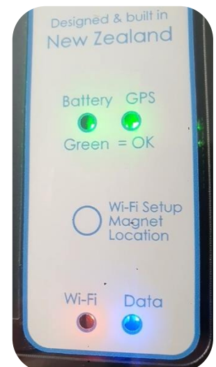
Lights visible on the deck unit.
