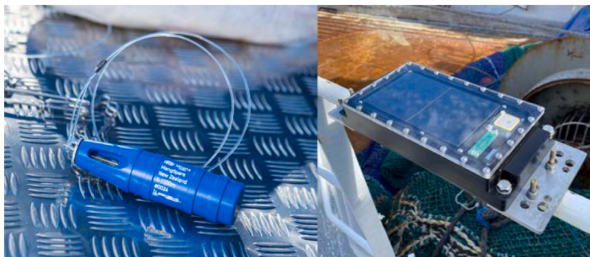
Fig. 3. The ZebraTech Moana TD1000 temperature and pressure sensor (left) and solar-powered deck unit (right).
