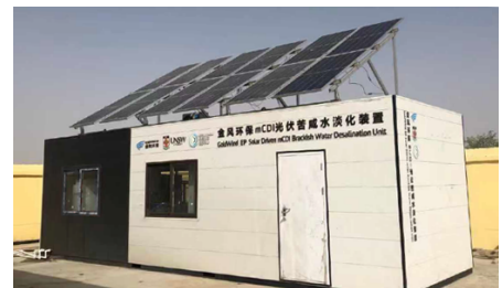
PV powered membrane CDI unit deployed in Xinjiang
