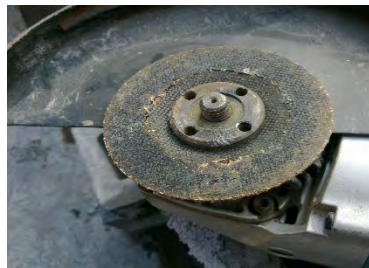
Damaged grinder disk being used on site
