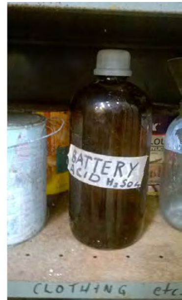
X – Wrong, improper labelling
