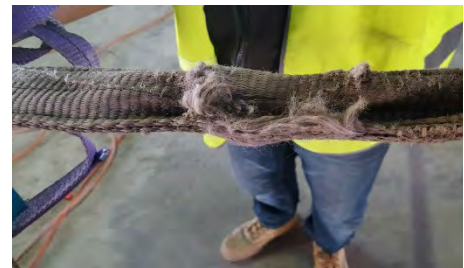
Damaged sling in use on site
