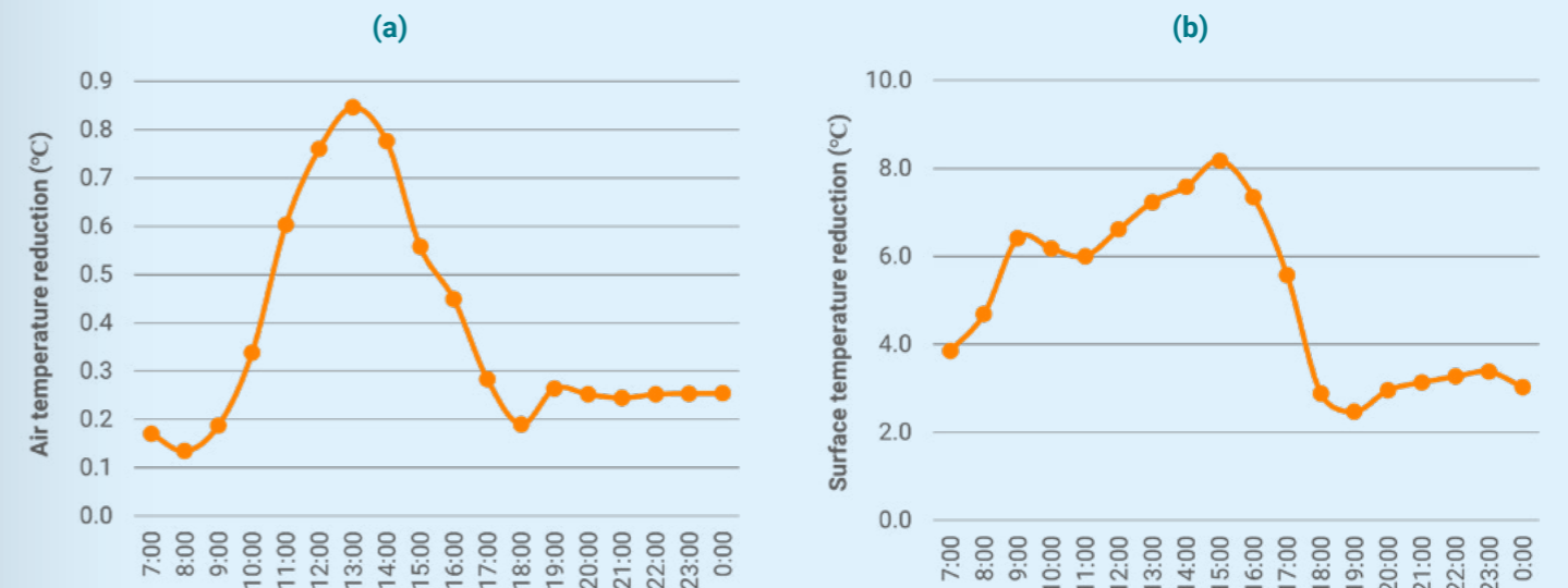
Figure C-37. Hourly maximum (a) air temperature and (b) surface temperature reductions from changing all lot sizes to 1,000 m 2 in Southlakes.
