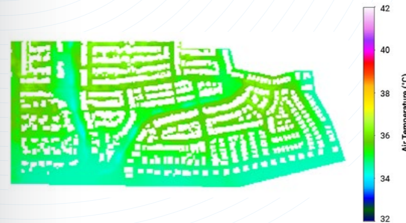
Figure C-21. Simulated air temperature distribution of the existing base case conditions of Southlakes at 2pm.
