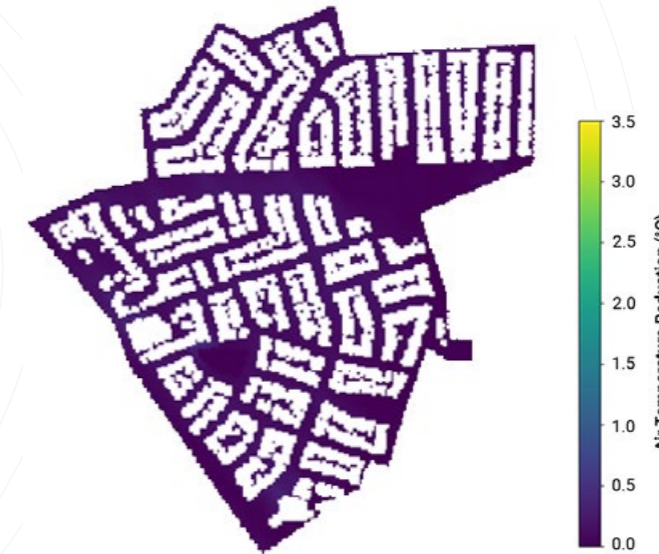
Figure B-29. Air temperature reduction distribution at 2pm from applying cool roofs to all buildings in Aberglasslyn.
