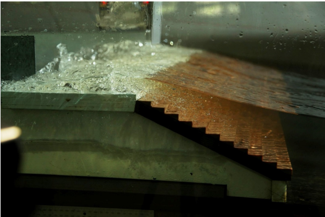
Figure 3: Stepped concrete seawall - Configuration C (5.45 m AHD Crest, no wave return wall) during 500 year ARI event, present day
