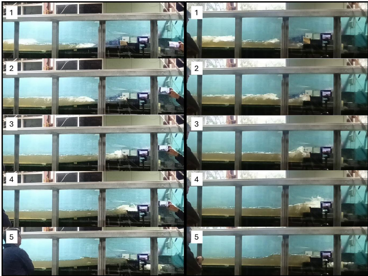
Figure 5.6 Image sequence comparison of V_{\max} event (13,000 L/m) for the accreted profile (left) [Test 2] and the V_{\max} event (20,300 L/m) for the eroded profile (right) [Test 1] with the Vertical Seawall with Wave Deflector structure subject to Design Condition 3
