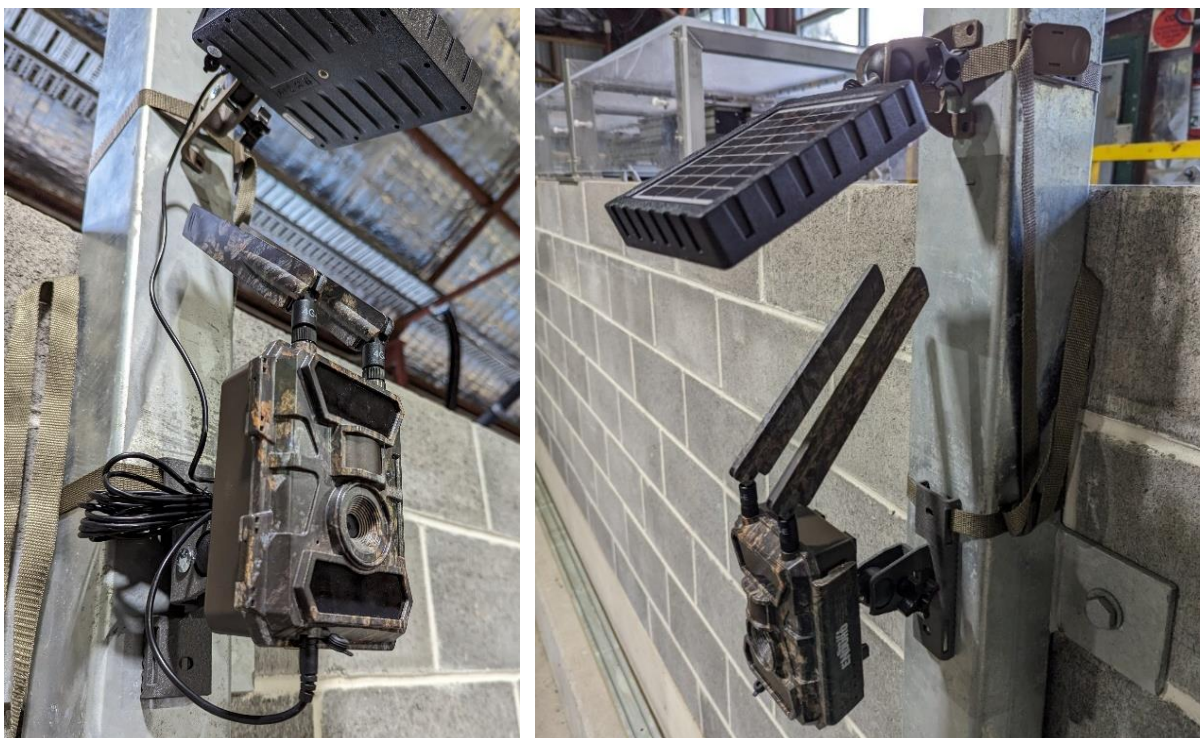
Figure 3.1 Photographs of an Enduro Swift 4G Trail Camera with solar panel prior to field deployment
