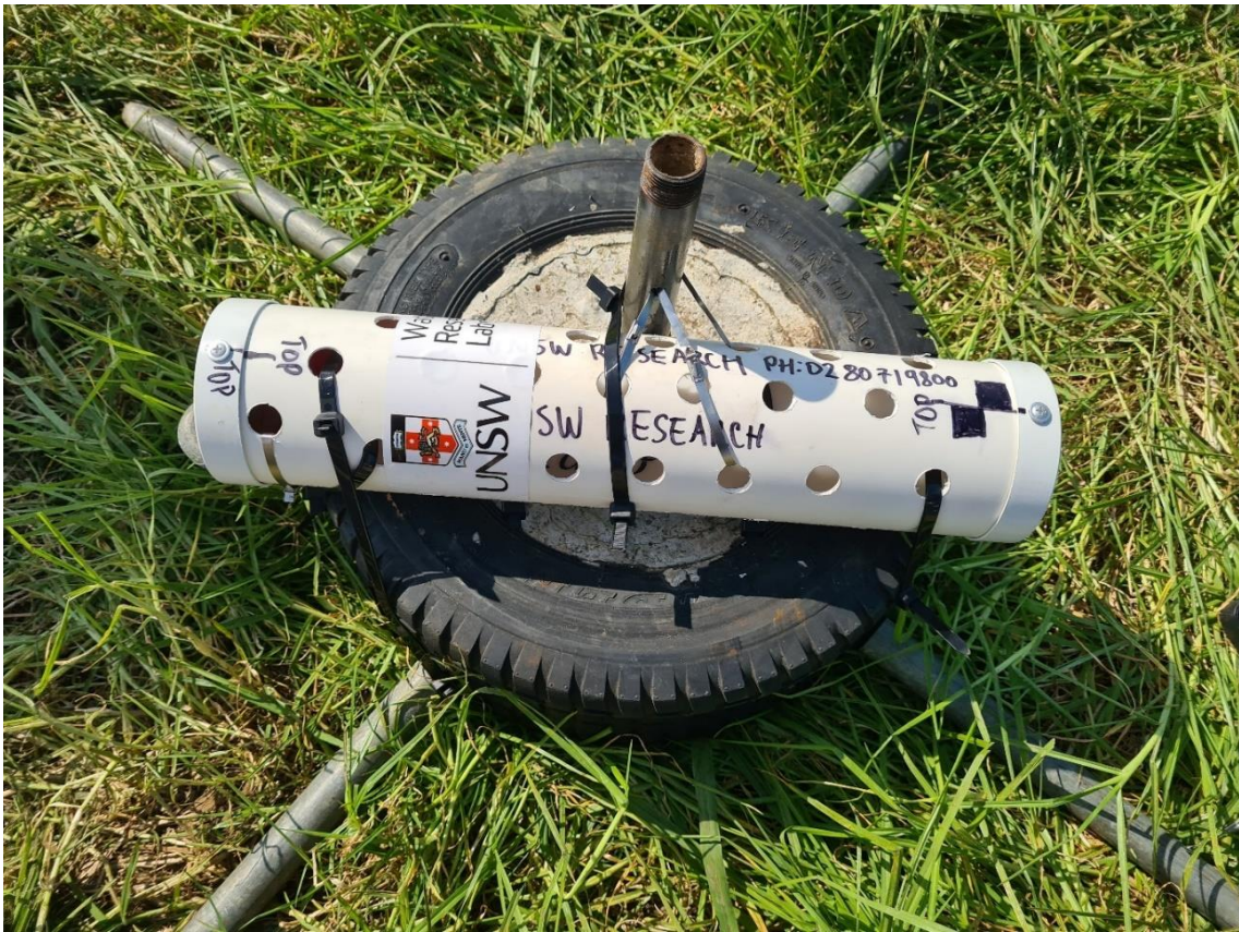
Figure 3.5 Photograph of portable wave probe mounting rig used in the Manning River
