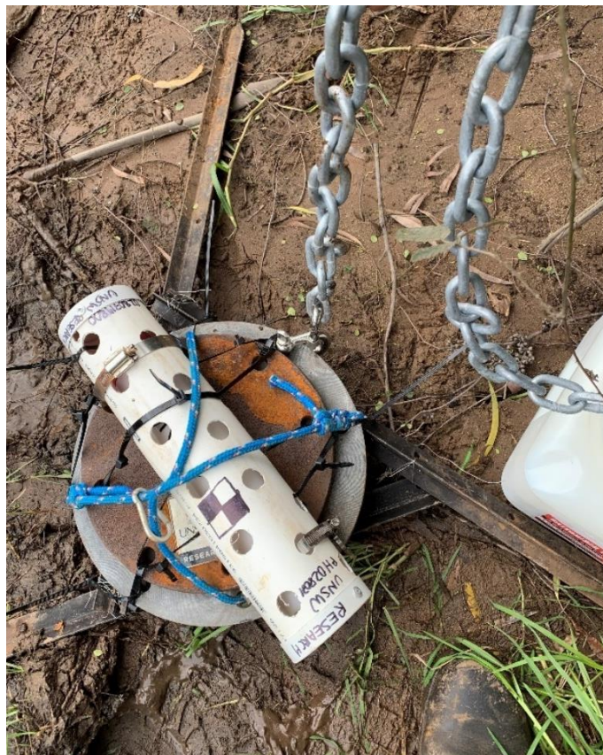
Figure 3.6 Photograph of portable wave probe mounting rig used in the Clyde River
