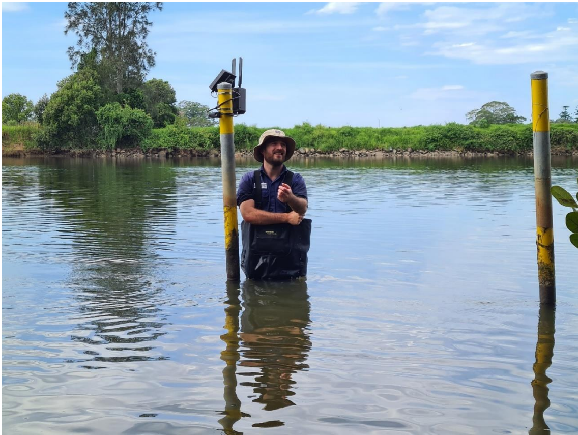
Figure 3.2 Photograph of camera and solar panel installed on the Manning River
