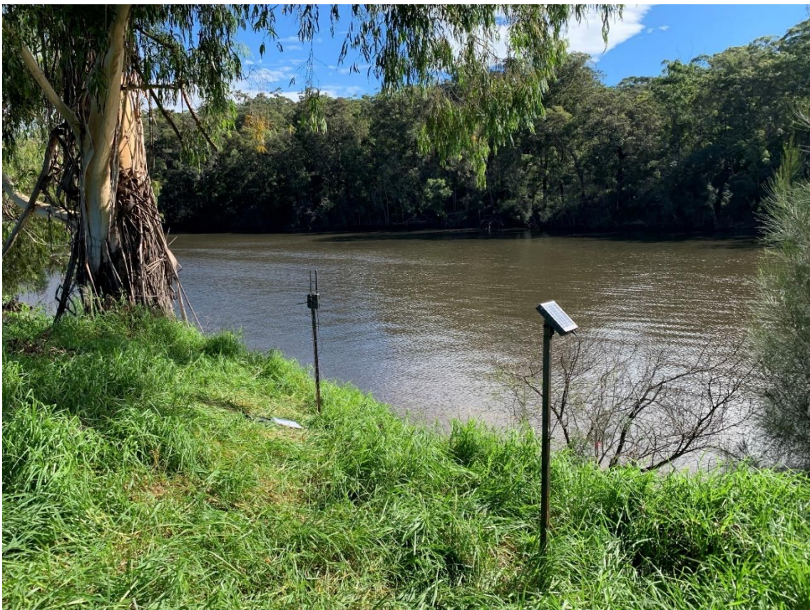
Figure 3.3 Photograph of camera and solar panel installed on the Clyde River
