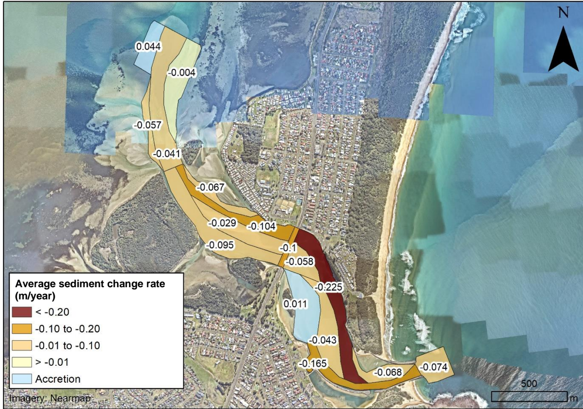
Figure 3.7 Average annual sediment change rate within each sediment compartment of the Lake Illawarra entrance channel (Tucker et al., 2023)
