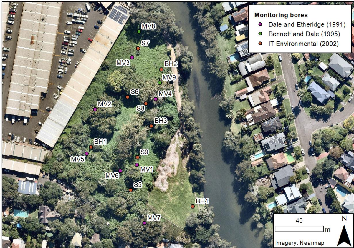
A.2: Historic monitoring bores at the Addiscombe Road remediation site
