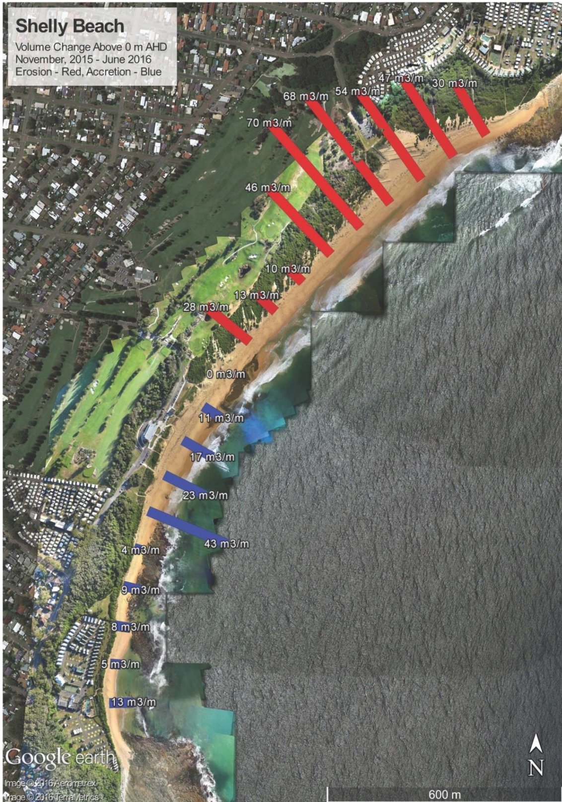
Figure 4-22: Volume change at Shelly Beach along several beach profiles
