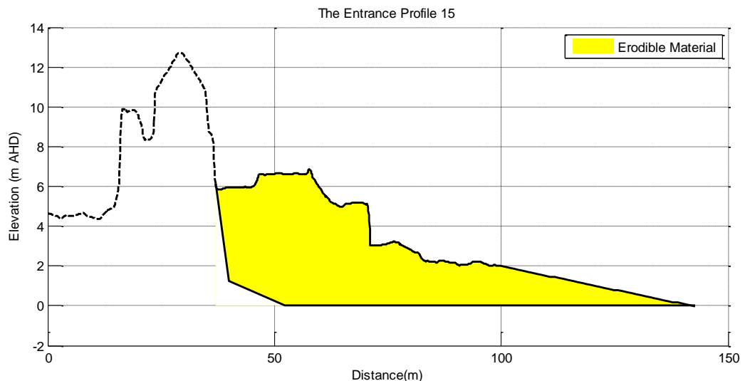
Figure 14: The Entrance North profile fronting property in the centre of Curtis Parade (Profile 15) showing volume of available sand buffer in the beach profile above 0 m AHD
