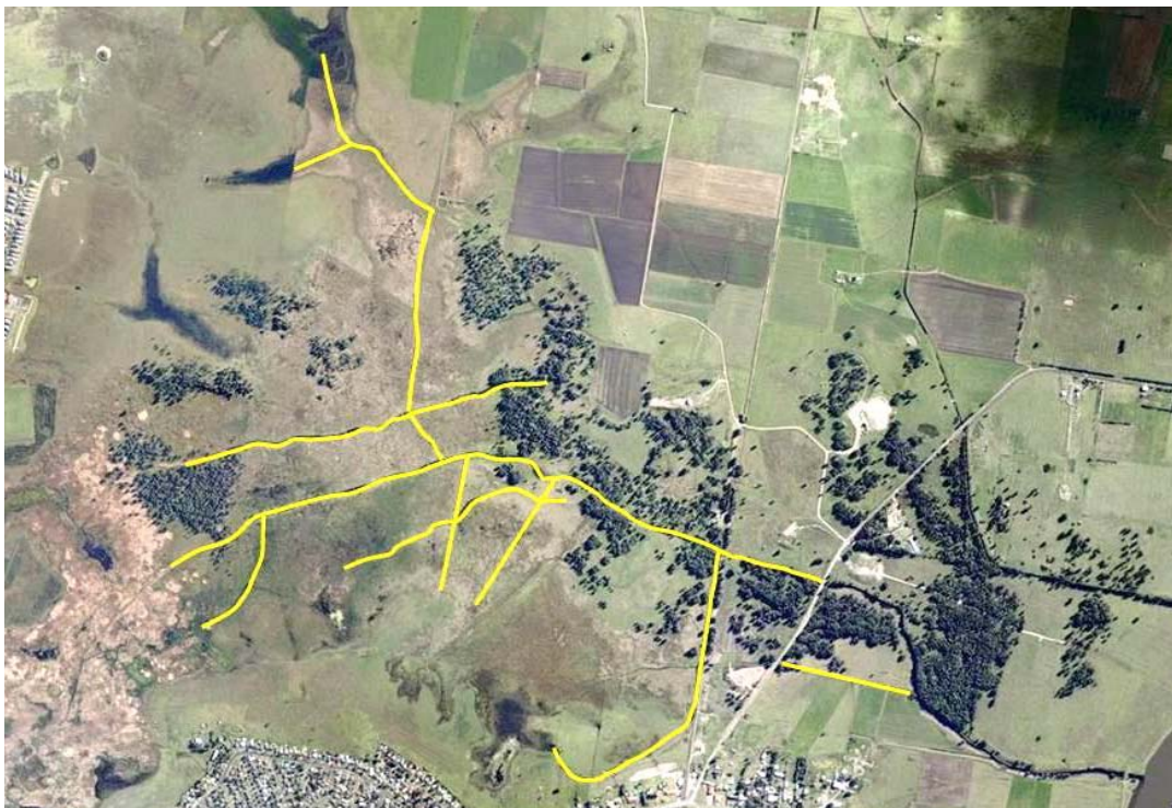
Figure 8.2: Identified drainage channels with significant in-drain vegetation
