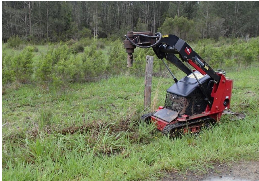
Figure F.4: Dingo Post Hole Digger Showing In-house Coupling used to Attach the Hand Auger
