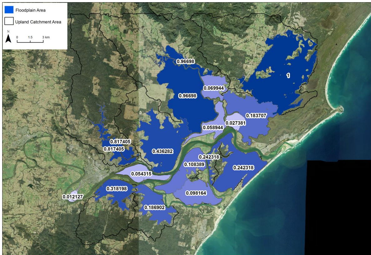
Figure D.3: Catchment Size Factor for Each Sub-Catchment of the Manning River Floodplain
