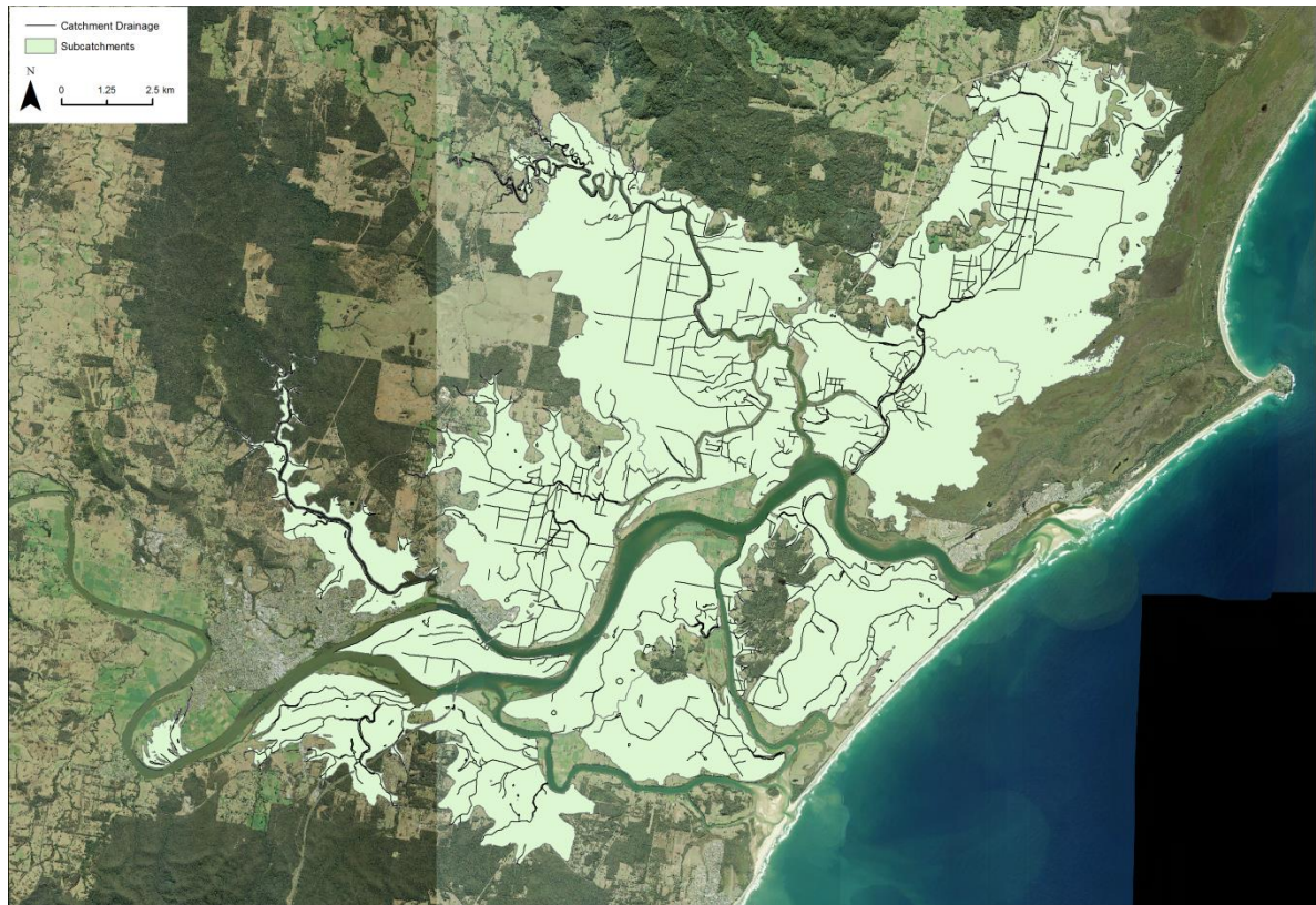
Figure C.5: Floodplain Drainage Network (Source: MidCoast Council)
