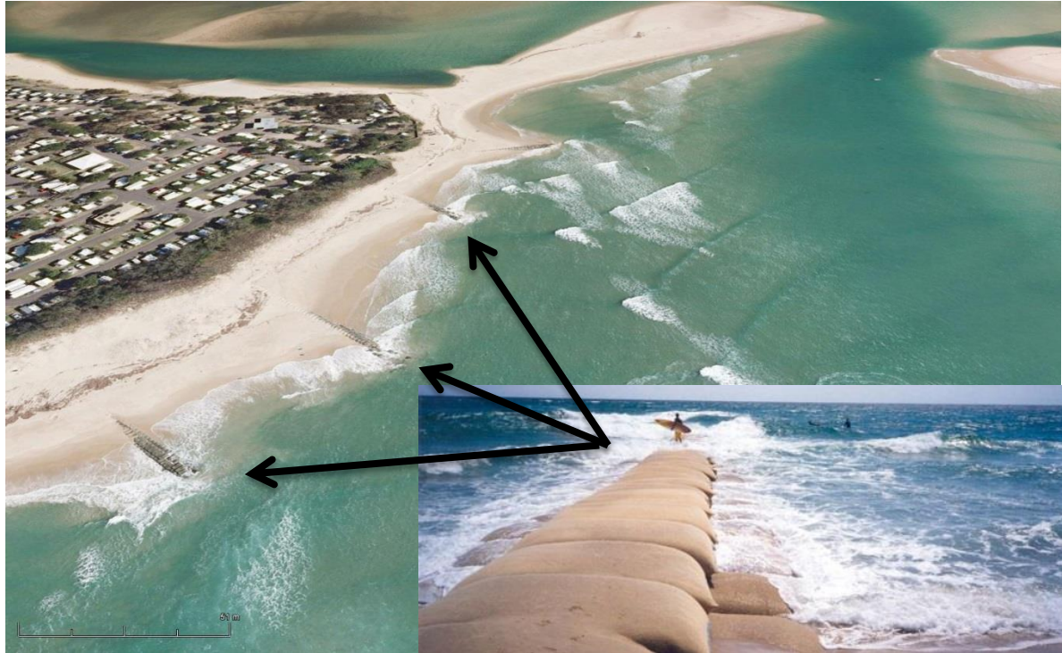
Figure 5.6. Maroochydore Geocontainer Groyne Design
