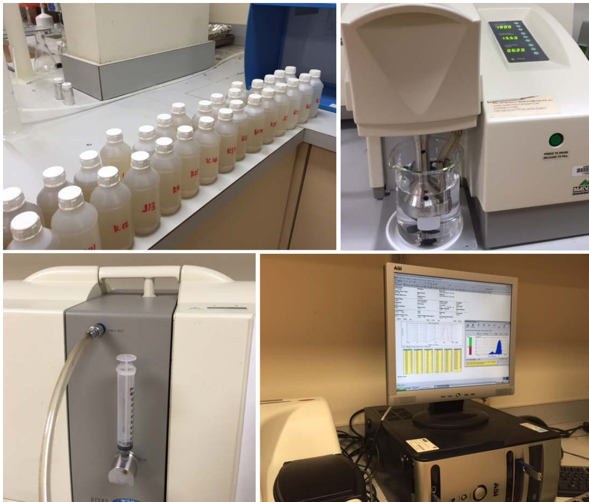
Figure 5-2: MasterSizer 2000 Particle Sampling Instrumentation Setup
