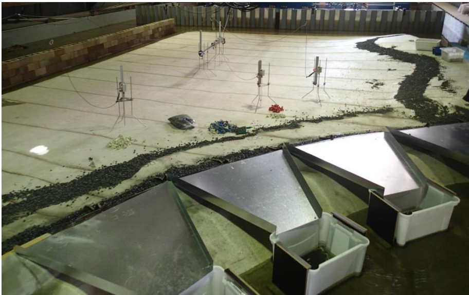
b) Overview of Existing Breakwater Core and of Muttonbird Island Shoreline with Increased Roughness
