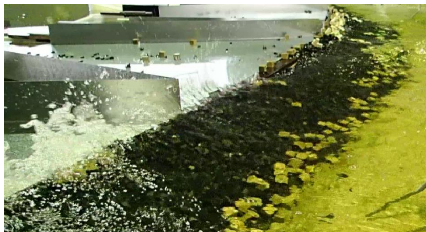
c) Overtopping Sequence from Ch. 650 m to Ch. 750 m with Displaced Concrete Cubes
