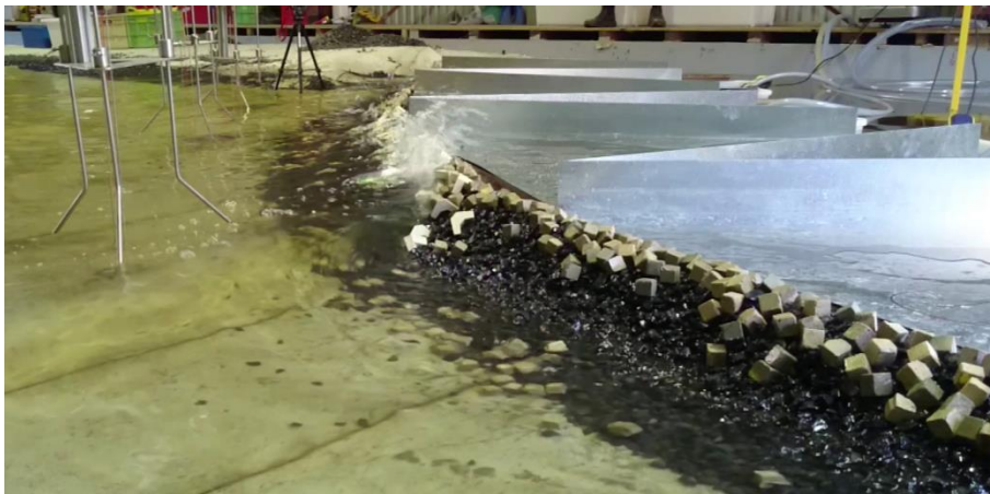
b) Example of Overtopping around Ch. 550 m
