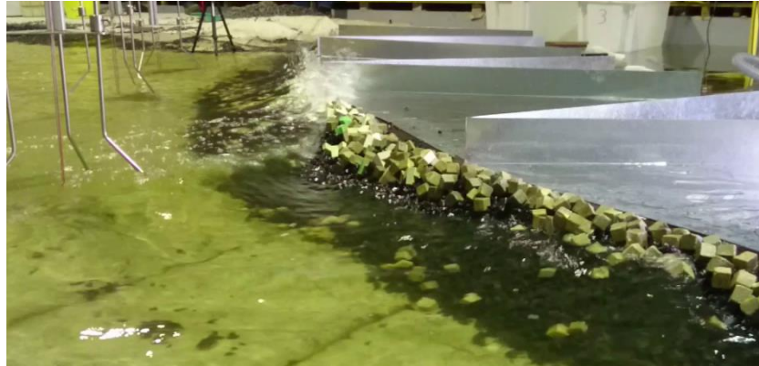
a) Simultaneous Green-Water Overtopping from Ch. 550 m to Ch. 600 m
