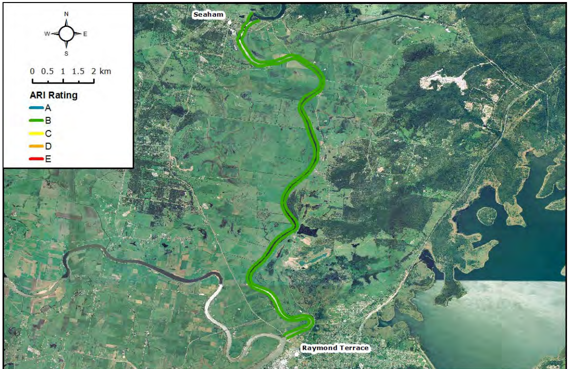
Figure K-7: Equivalent Wind/Boat Wave Average Recurrence Interval Rating - Wakeboard Operating - 8 Hour Duration – 10 Boat Passes (Lower Williams River)
