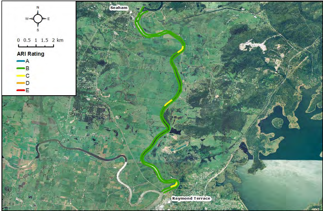
Figure K-11: Equivalent Wind/Boat Wave Average Recurrence Interval Rating - Waterski Operating - 8 Hour Duration – 50 Boat Passes (Lower Williams River)
