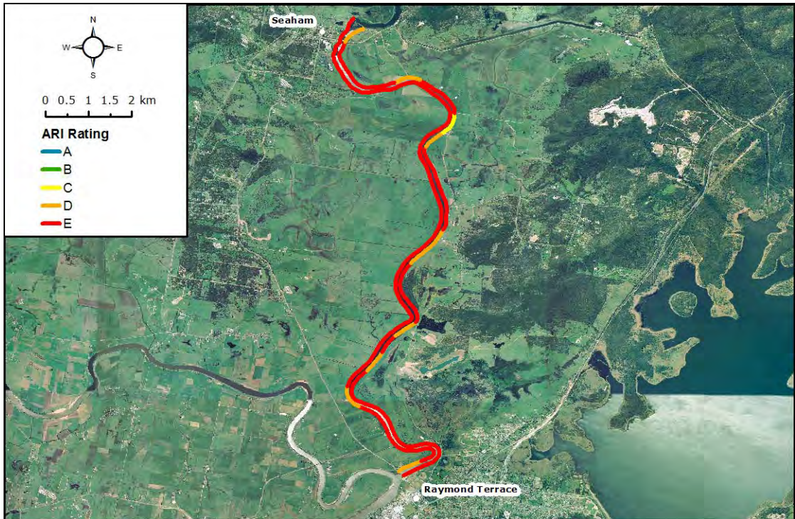
Figure K-15: Equivalent Wind/Boat Wave Average Recurrence Interval Rating - Wakesurf Operating - 8 Hour Duration – 150 Boat Passes (Lower Williams River)
