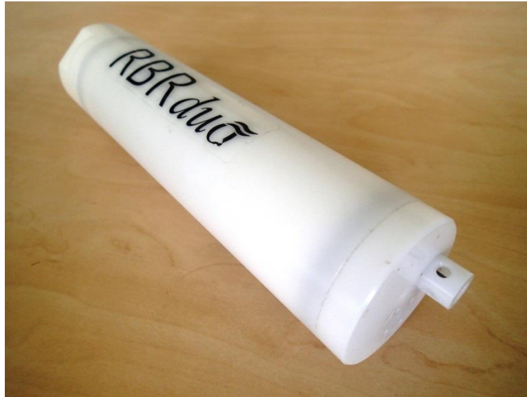
Figure D-2: RBRduo Wave Probe
