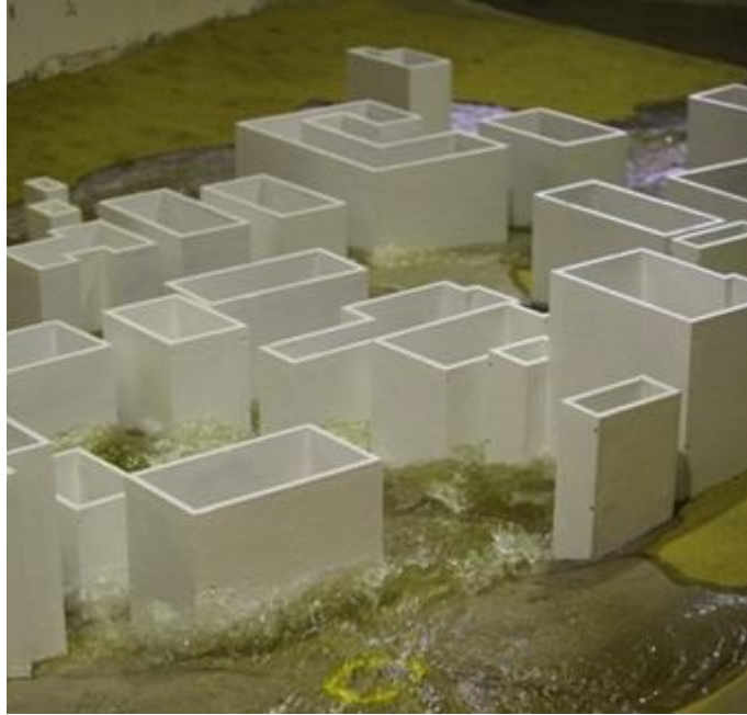
Figure 6-4: Merewether Heights physical model at WRL
