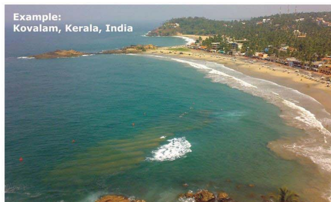
Figure 5.11 Nourishment with (Natural) End Control Structure and Offshore Breakwater (Submerged Reef)
