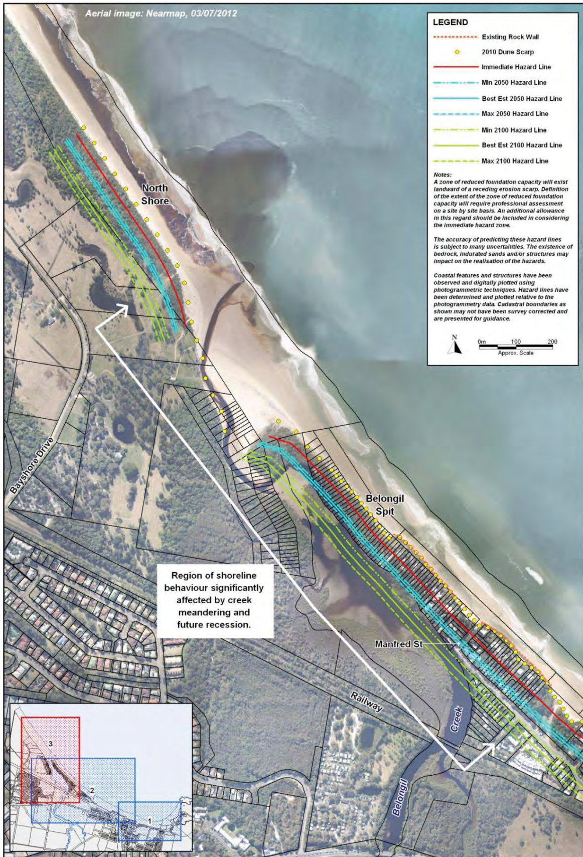
BMT WBM (2013) Figure A-8: Erosion Hazard Zones – Scenario 2 (Belongil Spit seawalls removed) Belongil Spit and Byron North Shore
