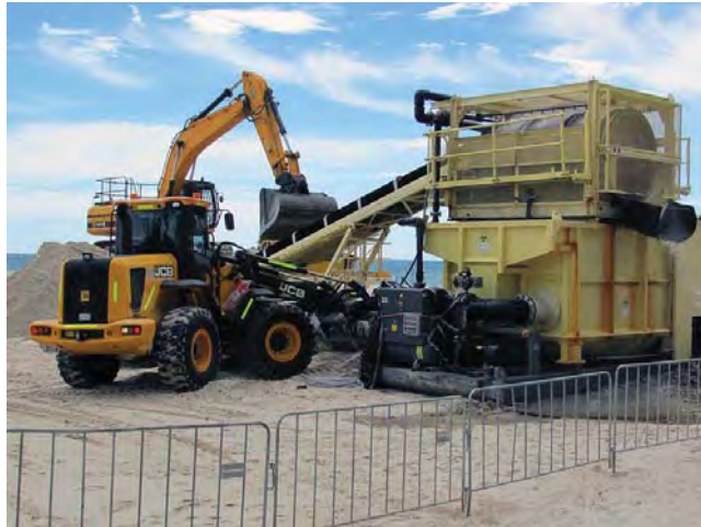
Figure 29.6: Mobile Sand Collecting Unit in Operation (Source: ABC Australia)
