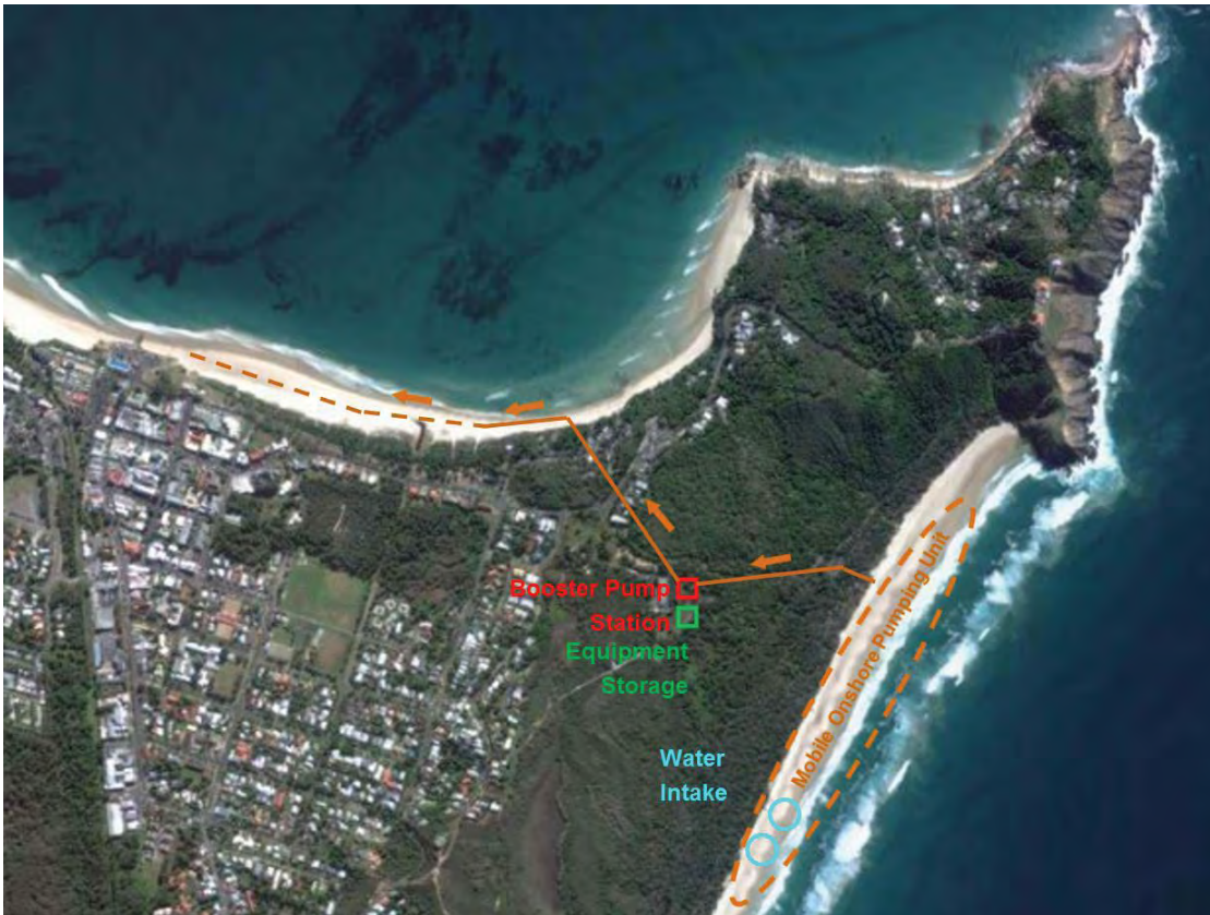
Figure 29.9: Schematic of a Possible Land-based Pumping System for Byron Bay
