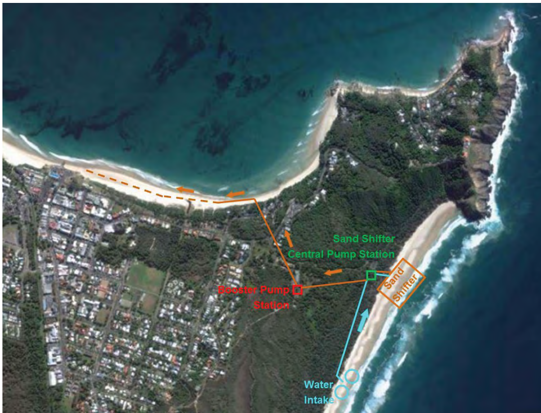
Figure 29.12: Schematic of a possible Sand Shifter System for Byron Bay
