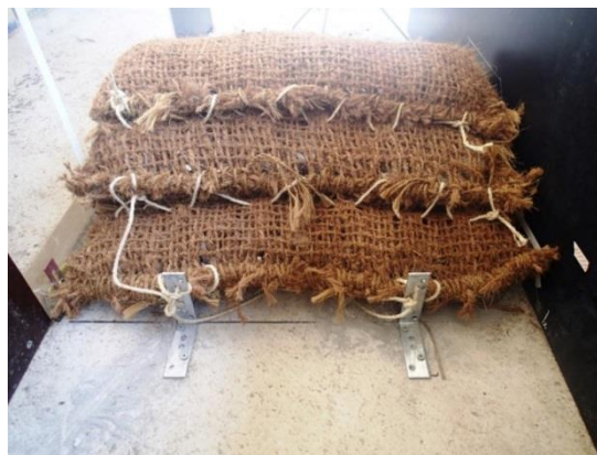
Figure 2.1 Three tier oyster shell filled bag arrangement - secured (Phase 2 tests)
