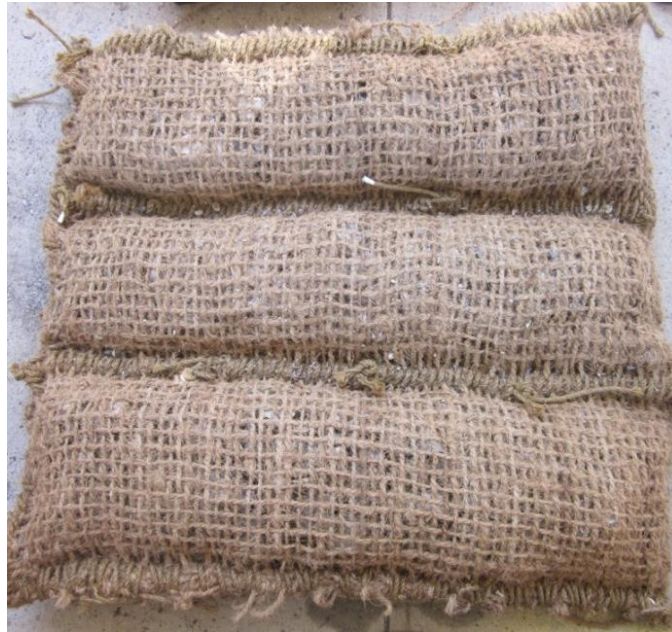
Figure 2.2 Example of triple oyster shell filled bag tested in the physical model
