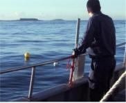
The field trials were undertaken by injecting the tracer under controlled conditions at the STP for a period of 4-6 hours. Based on predetermined calculations, the known concentration of Rhodamine WT was then diluted in the near-field. The extent of the dilutions was mapped using a fluorimeter attached to a Seabird 19Plus, a differential GPS and a range of sampling equipment
