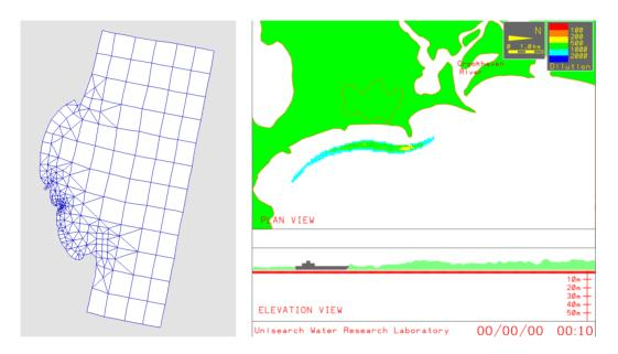
Hydrodynamic modelling was primarily undertaken with a depth averaged mesh, using RMA 10. Limited three-dimensional simulations were also undertaken to show the impact of winds on near-surface currents (and therefore transport of surface plumes). The model was calibrated against current data recorded by a moored ADCP near the site and later verified against ADCP transects collected near the sites of interest.
