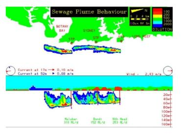
A three dimensional modelling suite was established specifically for modelling around the Sydney outfalls, including three discrete components: a near-field model (PLUMEL2), a 3D hydrodynamic far-field model (RMA10) and a far-field water quality model (3DRWALK). The monitored data is input into these models to predict plume behaviour. WRL provides numerical modelling of the outfall plumes in 3D and supplies the results to Sydney Water via the internet.
