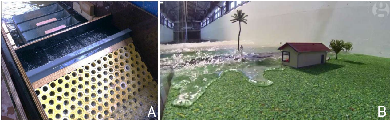
Fig. 15: Example wave flume testing setups at the University of New South Wales - Water Research Laboratory showing A) a wave deflector and back beach washout zone with overtopping collection trays and B) a wave flume model of storm surge impacts on island reef coastlines under different climate change and sea level rise scenarios.
