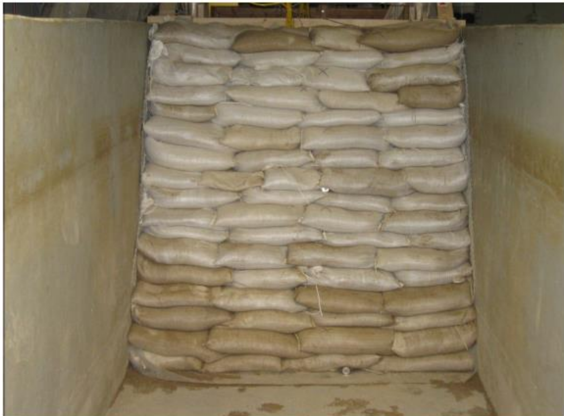
Figure 2.8 - Front face of sandbag dike using woven slit film polypropylene (WSFPP) (Offman 2009)
