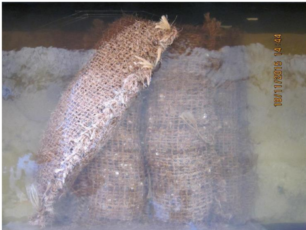
Figure 2.4 - Before and after photos illustrating complete displacement of the crest oyster bag during wave testing (Coghlan et al. 2016)
