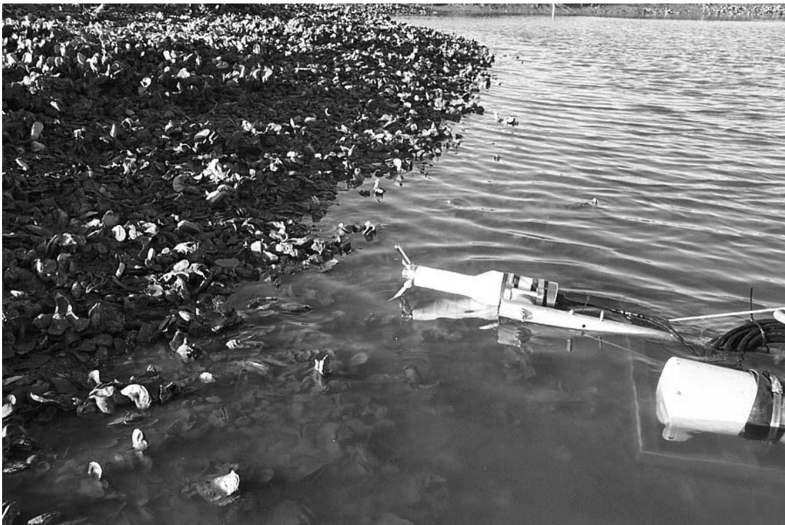
Figure 2.6 – Intertidal channel oyster bank with ADV probe positioned on the lower bank (Styles 2015)
