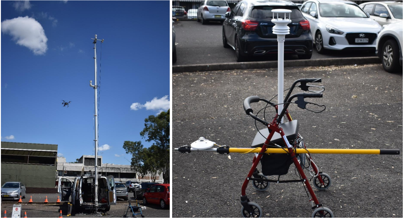
Figure 9. Energy Bus and drone (left) and cart with pyranometer and weather station (right).
