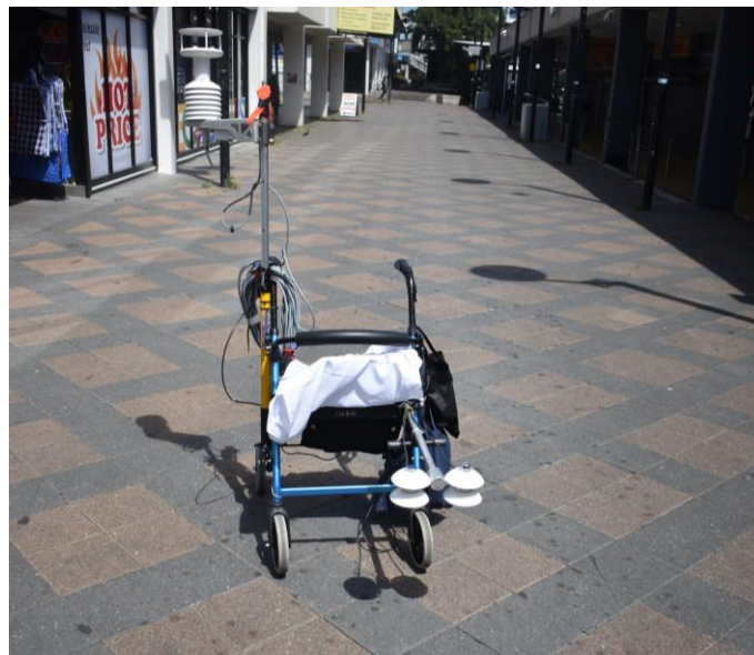
Figure 12. Cart equipped with a net radiometer, shown while performing measurements along Dawson Mall.
