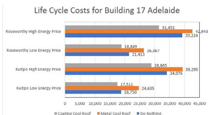
Figure 12. Life Cycle Costs for Building 17 for Kuitpo and Roseworthy weather stations.
