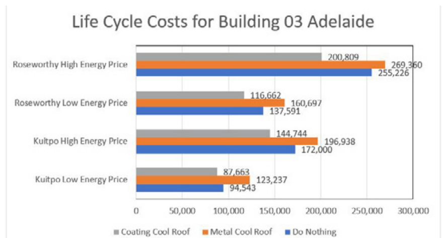
Figure 12. Life Cycle Costs for Building 03 for Kuitpo and Roseworthy weather stations.
