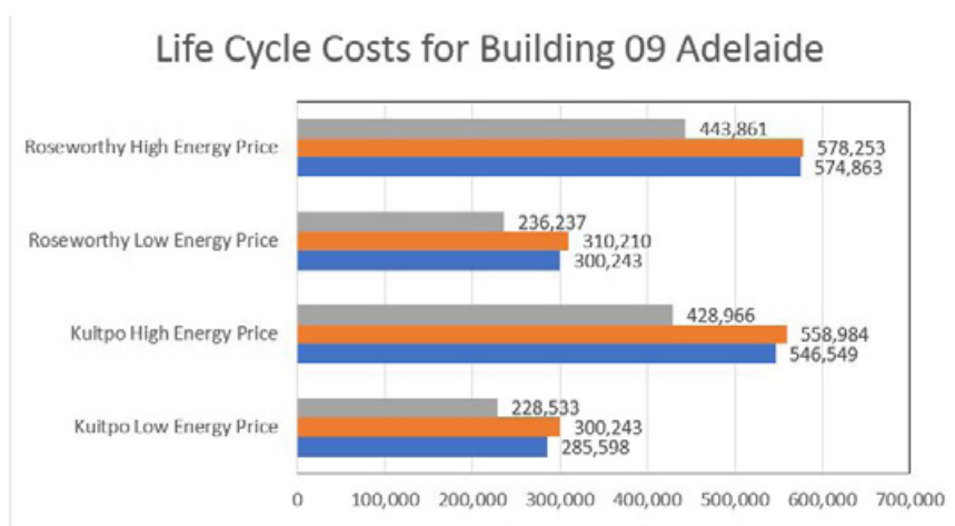
Figure 12. Life Cycle Costs for Building 09 for Kuitpo and Roseworthy weather stations.
