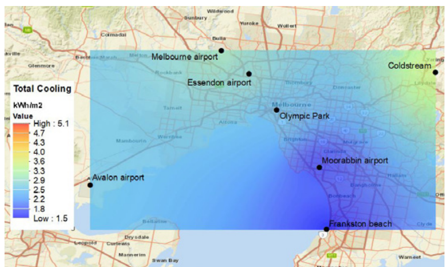
Figure 3. Spatial distribution of total cooling load for cool roof with modified urban temperature scenario (scenario 2) for two summer months (i.e. January and February) for a new mid-rise apartment building with weather data simulated by WRF for COP=1 for heating and cooling.
