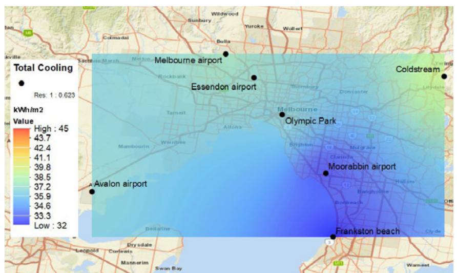
Figure 3. Spatial distribution of total cooling load for cool roof with modified urban temperature scenario (scenario 2) for two summer months (i.e. January and February) for a new mid-rise shopping mall centre with weather data simulated by WRF for COP=1 for heating and cooling.
