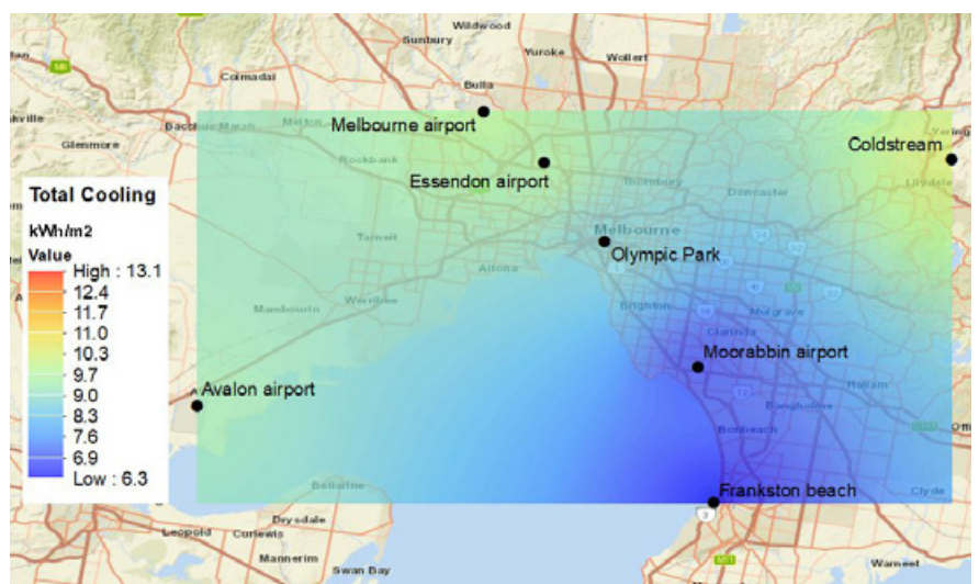
Figure 3. Spatial distribution of total cooling load for cool roof with modified urban temperature scenario (scenario 2) for two summer months (i.e. January and February) for an existing school with weather data simulated by WRF for COP=1 for heating and cooling.
