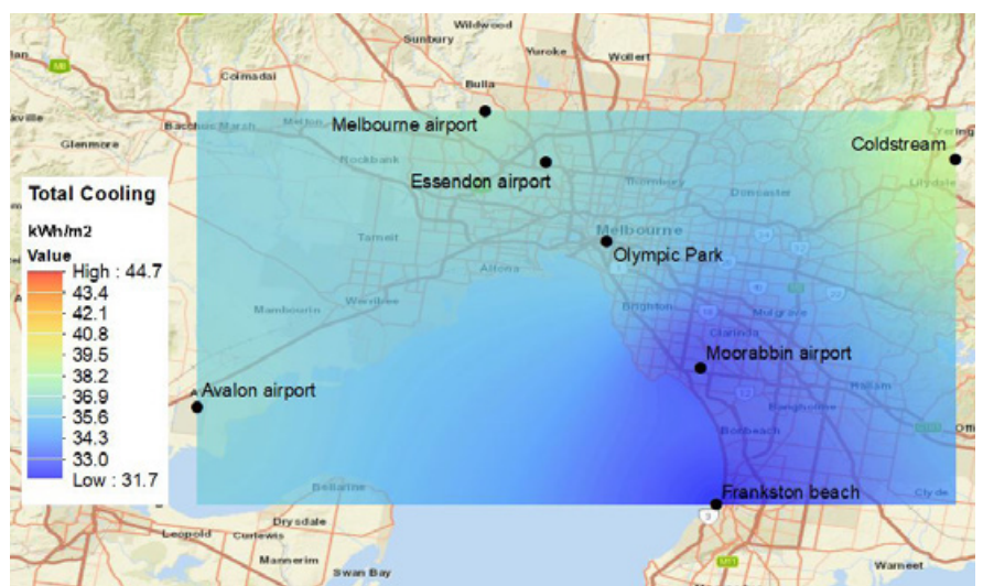
Figure 3. Spatial distribution of total cooling load for cool roof with modified urban temperature scenario (scenario 2) for two summer months (i.e. January and February) for a new high-rise shopping mall centre with weather data simulated by WRF for COP=1 for heating and cooling.
