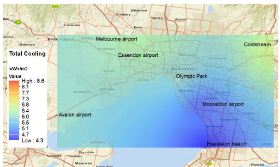
Figure 3. Spatial distribution of total cooling load for cool roof with modified urban temperature scenario (scenario 2) for two summer months (i.e. January and February) for a low-rise office building without insulation with weather data simulated by WRF for COP=1 for heating and cooling.
