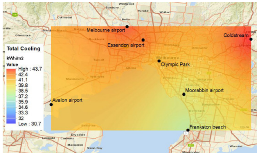
Figure 2. Spatial distribution of total cooling load for reference with cool roof scenario (scenario 1) for two summer months (i.e. January and February) for an existing high-rise shopping mall centre with weather data simulated by WRF for COP=1 for heating and cooling.
