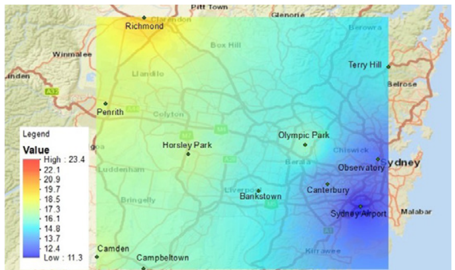
Figure 3. Spatial distribution of total cooling load for cool roof with modified urban temperature scenario (scenario 2) for two summer months (i.e. January and February) for a new high-rise office building with insulation with weather data simulated by WRF for COP=1 for heating and cooling.
