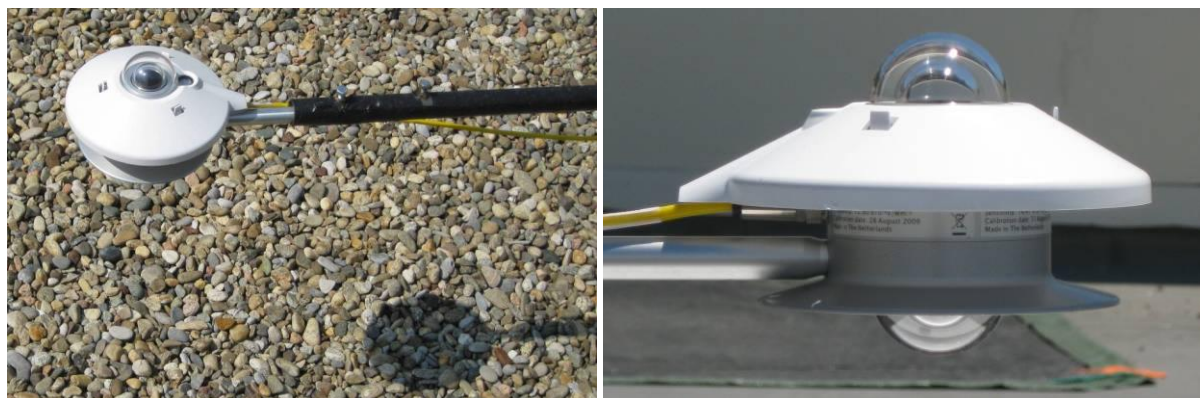
Figure 17 An albedometer measuring a gravel roof. On the right, the detail of the two domes is shown.
