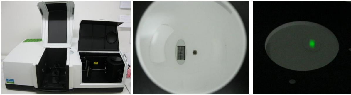
Figure 15 Spectrophotometer with an integrating sphere, with a detail of the photomultiplier and PMT detector (in this case) at the bottom of the sphere and then the measurement beam at the reflectance port.
