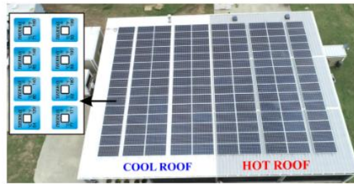
Figure 11 THERMAX technique (Thermax®) for thermal evaluation of the Rubicon buildings' roofs. (Rahmani et al., 2021)
