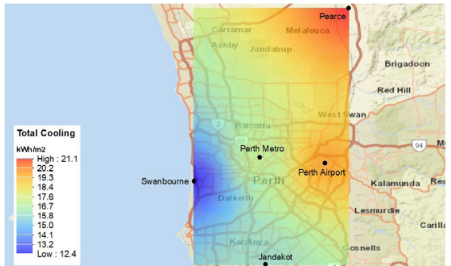
Figure 1. Spatial distribution of total cooling load for reference scenario for two summer months (i.e. January and February) for a new low-rise office building with roof insulation with weather data simulated by WRF for COP=1 for heating and cooling.
