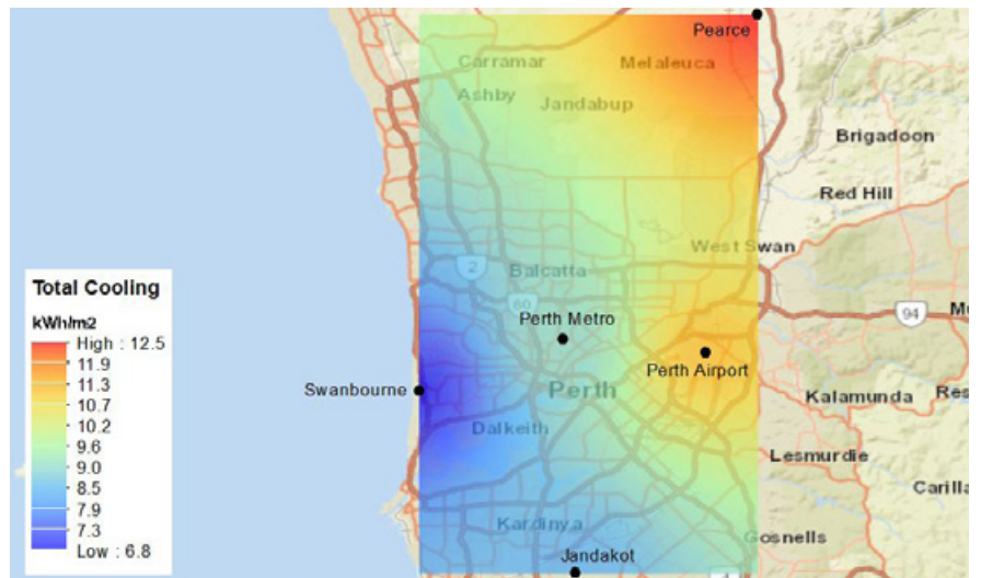
Figure 1. Spatial distribution of total cooling load for reference scenario for two summer months (i.e. January and February) for a new high-rise apartment building with weather data simulated by WRF for COP=1 for heating and cooling.
