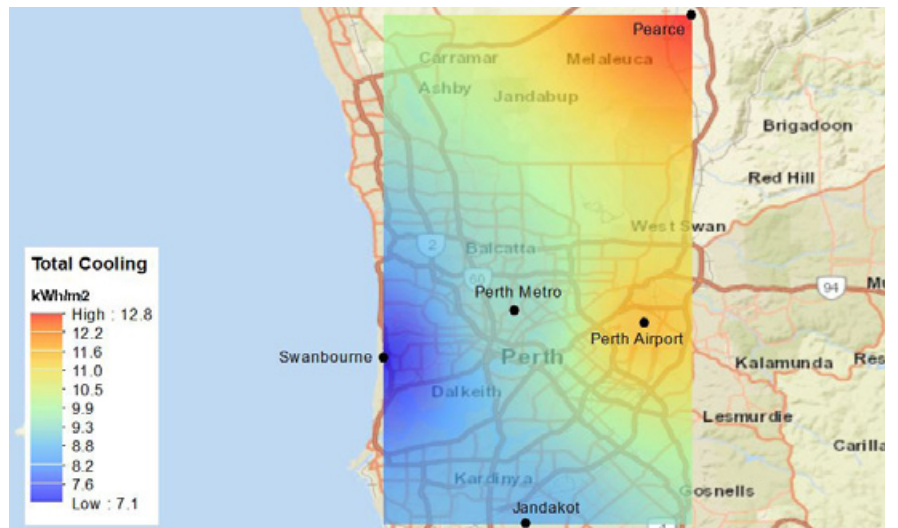
Figure 1. Spatial distribution of total cooling load for reference scenario for two summer months (i.e. January and February) for a new mid-rise apartment building with weather data simulated by WRF for COP=1 for heating and cooling.
