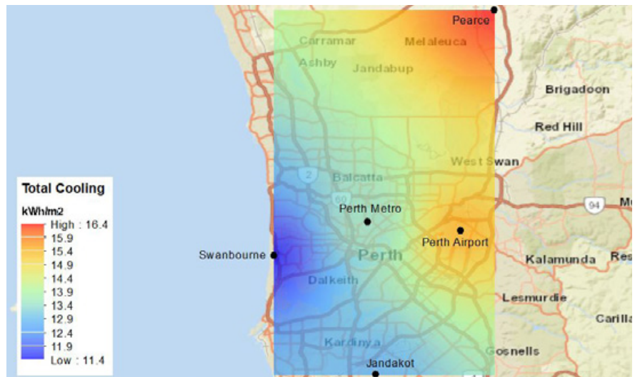
Figure 1. Spatial distribution of total cooling load for reference scenario for two summer months (i.e. January and February) for a typical existing stand-alone house with weather data simulated by WRF for COP=1 for heating and cooling.
