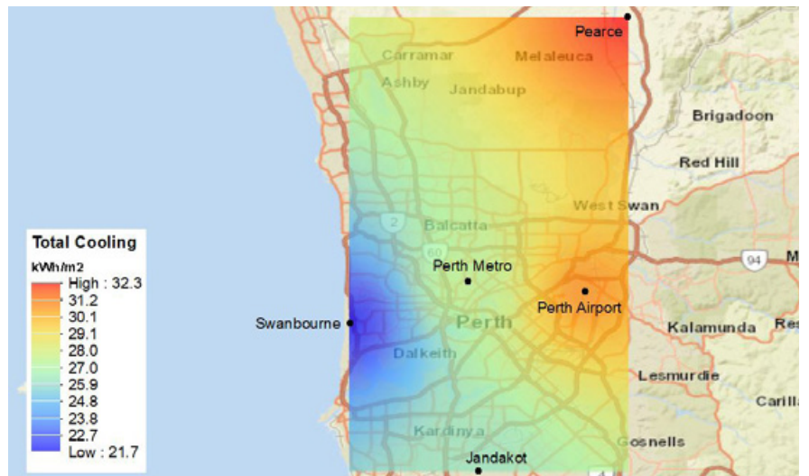
Figure 1. Spatial distribution of total cooling load for reference scenario for two summer months (i.e. January and February) for a low-rise office building without insulation with weather data simulated by WRF for COP=1 for heating and cooling.
