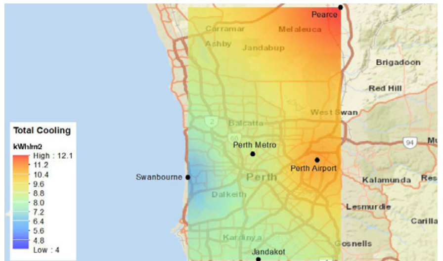
Figure 2. Spatial distribution of total cooling load for reference with cool roof scenario (scenario 1) for two summer months (i.e. January and February) for a new high-rise apartment building with weather data simulated by WRF for COP=1 for heating and cooling.
