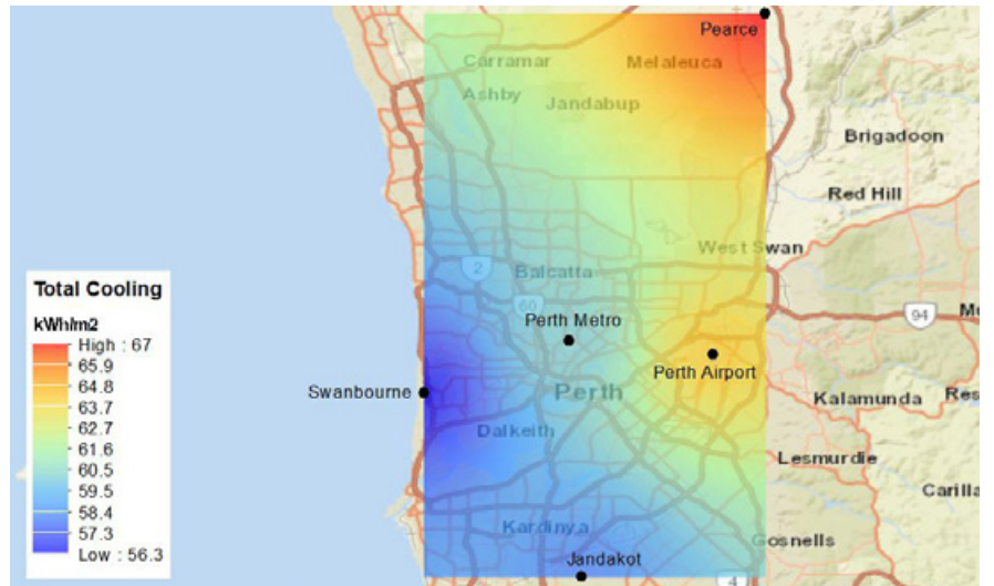
Figure 1. Spatial distribution of total cooling load for reference scenario for two summer months (i.e. January and February) for a new high-rise shopping mall centre with weather data simulated by WRF for COP=1 for heating and cooling.
