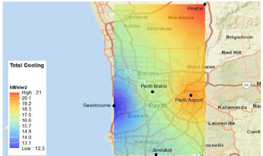
Figure 1. Spatial distribution of total cooling load for reference scenario for two summer months (i.e. January and February) for an existing high-rise office building with insulation with weather data simulated by WRF for COP=1 for heating and cooling.
