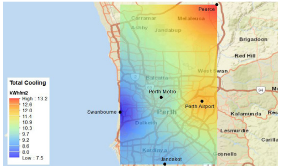
Figure 1. Spatial distribution of total cooling load for reference scenario for two summer months (i.e. January and February) for a new low-rise apartment building with weather data simulated by WRF for COP=1 for heating and cooling.
