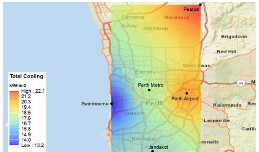
Figure 1. Spatial distribution of total cooling load for reference scenario for two summer months (i.e. January and February) for a high-rise office building without insulation with weather data simulated by WRF for COP=1 for heating and cooling.
